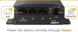
Power the device normally through Power over Ethernet for less cable management, or an industrial microfit connector for a secure and durable power option.
