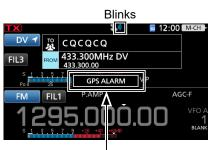
"GPS ALARM" pops up on the screen and the alarm sounds 3 times.
