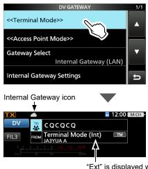
"Ext" is displayed when using the External Gateway function.
