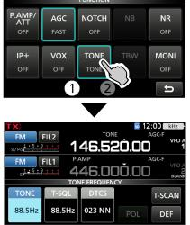
3. Rotate (MAIN DIAL) to select the desired subaudible tone frequency.
