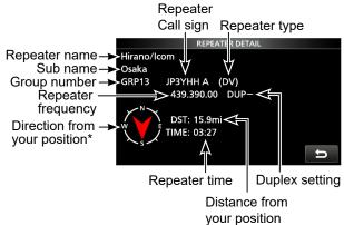
\* When the "POSITION" setting (p. 11-30) is set to "Approximate" on the repeater list, the direction data is not displayed if the distance to the repeater is less than 5 kilometers.
