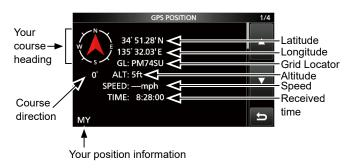
When the "GPS Select" is set to "Manual," SPEED, Compass and Compass Direction are not displayed.
