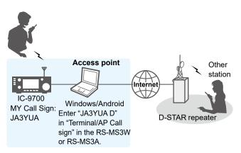
Before using the DV Gateway function, you have to set up a network.
