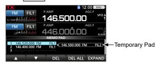
**TIP:** If you change the frequency or operating mode called up from Memo Pads, the contents are automatically updated in a temporary Pad.
