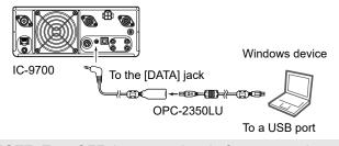
**NOTE:** Turn OFF the transceiver before connecting or disconnecting the cable.
