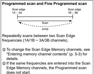
The Fine Programmed scan is most effective in the SSB, CW, and RTTY modes.
