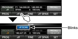
① When a signal is detected, the scan pauses according to the "SCAN Resume" setting, and then resumes.
