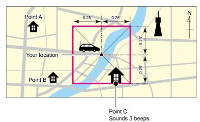
Alarm Area (RX/Memory) (Setting specific station) When a specific GPS Memory is selected:
