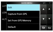
**TIP:** When you select "Capture From GPS" or "Set From GPS Memory," you can capture the position from the GPS, or set the Object's position from the GPS memory.
