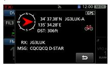
When you receive the signal, the RX position data is displayed in the RX position window.
