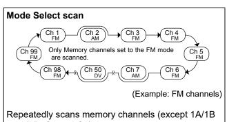
Repeatedly scans memory channels (except 1A/1B ~ 3A/3B, C1 and C2) that are set to the mode selected before starting the scan.
