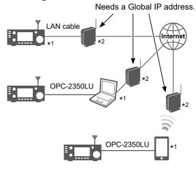
\*1 A static IP address to the transceiver, Windows, or Android device is recommended.
