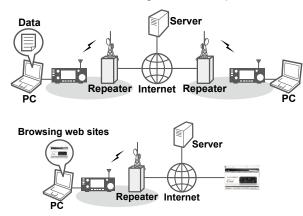
While in the DD mode and the "TX INHIBIT" is set to "OFF," the data is automatically sent when data is input from a PC. The received data is output on the PC.
