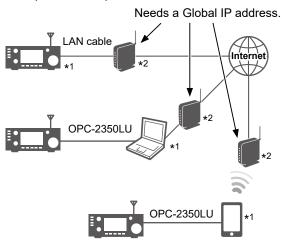
\*1 A static IP address to the transceiver, Windows, or Android device is recommended.
