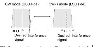
**TIP:** Reversing the carrier point The carrier point of the CW mode is USB by default. You can change it to LSB on the FUNCTION screen.
