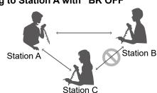
Station B does not hear that Station C is calling Station A.
