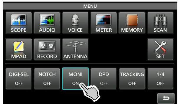
5. Rotate [MULTI] to adjust MONITOR to the clearest audio output between 0% and 100%, while speaking at your normal voice level.
