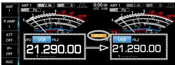
3. While holding down **[XFC]**, set the operating frequency offset between transmit and receive.
