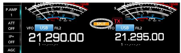
4. Touch the Main band's frequency readout to return to receive on the Main band.
