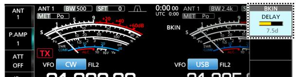
4. Rotate **MULTI** to set to where the transceiver does not return to receive while keying.
