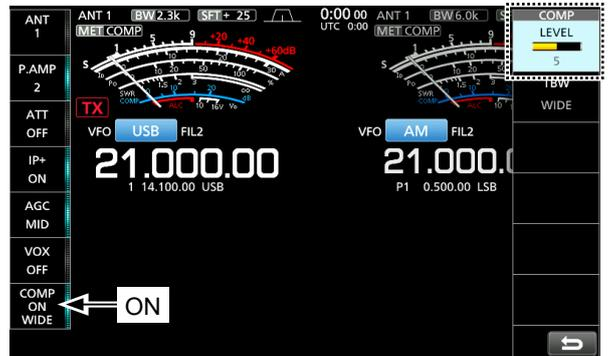
8. While speaking into the microphone at your normal voice level, adjust the Speech Compressor level to where the COMP meter reads within the COMP zone (10 to 20 dB range).
