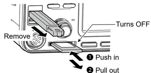
① Push in the SD card until a click sounds to unlock the card and to pull it out.
