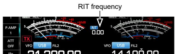
2. Rotate [RIT/ATX] to set the RIT frequency to match the transmitting station's frequency.
