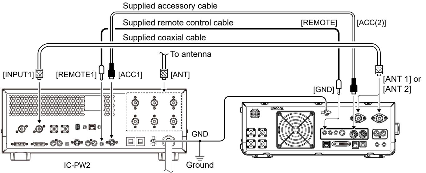
**⚠ WARNING!** When using a linear amplifier such as the IC-PW2, set the RF POWER in the Multi-function menu to keep the ALC meter in the red zone.
