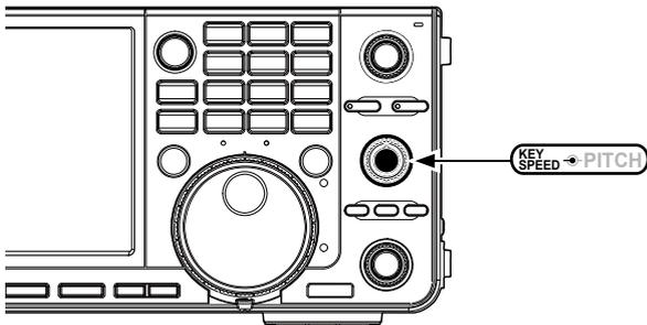
• The keying speed is displayed under the time display while setting.
