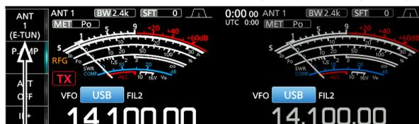
(E-TUN): The internal tuner is ON in the Emergency mode.
