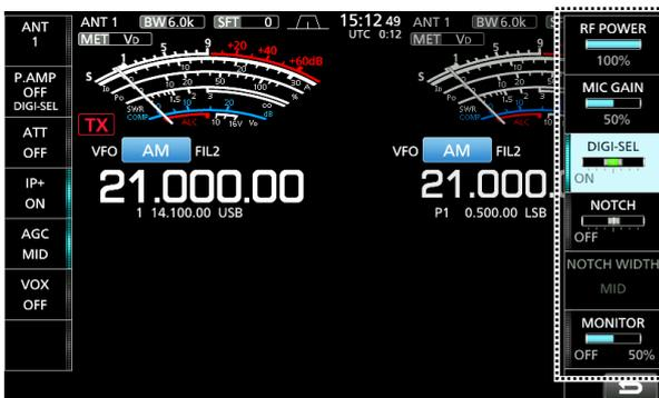
2. Rotate **[MULTI]** to adjust the center frequency.
