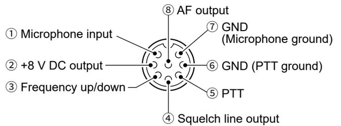
**NOTE:** Pin 1 outputs 8 V DC power for Icom microphones.
