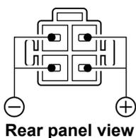
Accepts the regulated DC power for 13.8 V DC ±15% through the supplied DC power cable.
