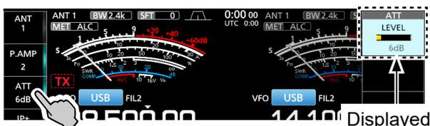
2. Rotate [MULTI] to adjust the attenuator level of up to 45 dB.
