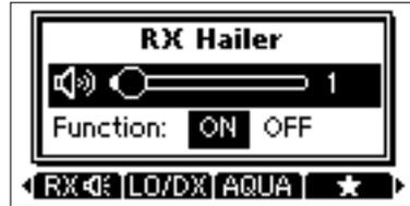
3. Push **▲**, and then push **◀** or **▶** or rotate **[DIAL]** to adjust the volume level.
