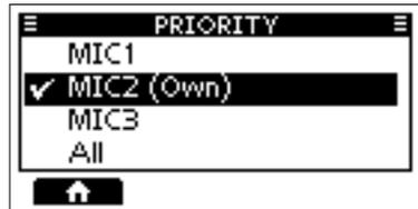
2. Push [▲] or [▼], or rotate [DIAL] to select a controller to be used as the Priority Controller.
