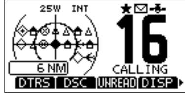
**NOTE:** An alarm sounds when an AIS target is closer than the CPA (Closest Point of Approach) and TCPA (Time to CPA) settings, and so on, depending on the presetting. To stop the alarm buzzer, push any key.
