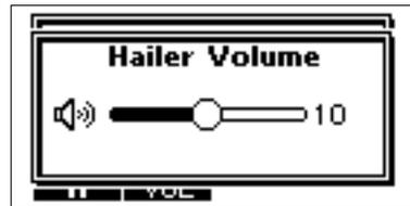
**NOTE:** While in the Hailer mode, the transmit and receive functions are disabled. When the transceiver is transmitting, the Hailer function is disabled.
