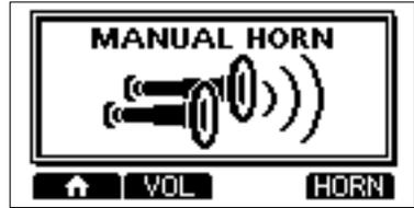
**NOTE:** While in the Horn mode, the transmit and receive functions are disabled. When the transceiver is transmitting, the Horn function is disabled.
