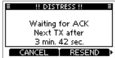
6. When you receive an Acknowledgment, an alarm sounds. Push **ALARM OFF** to turn OFF the alarm.
