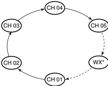
\*For the USA version, when the Weather Alert function is ON, the previously selected Weather channel is also scanned.
