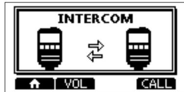
4. After releasing **CALL**, hold down [PTT] and speak into the microphone at your normal voice level.
