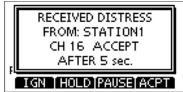
**ACPT:** Accepts the call. Channel 16 is automatically selected. Monitor Channel 16 as a coast station may require assistance. After Channel 16 is selected, select your next operation by pushing the Software Key below the following options.
