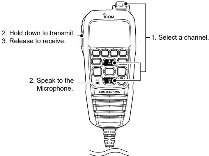
**TIP:** To maximize the readability of your transmitted signal, pause for a second after holding down [PTT] and hold the microphone 5 to 10 cm from your mouth, and then speak at your normal voice level.
