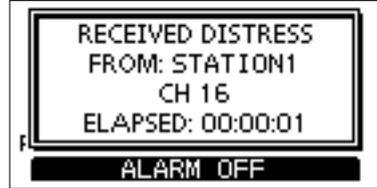
1. Push **ALARM OFF** to turn OFF the alarm.
