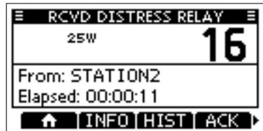
5. Push **CALL** to send the Distress Relay acknowledgment.
