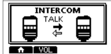
**NOTE:** While in the Intercom mode, the transmit and receive functions are disabled. When the transceiver is transmitting, the Intercom function is disabled.
