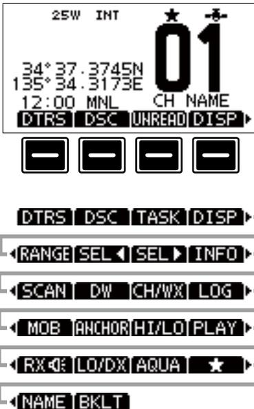
**NOTE:** The displayed icons or their order may differ, depending on the transceiver version or the presetting. When the MMSI code is not set, the Software Keys for the DSC function are not displayed.
