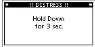
4. While lifting up the key cover, hold down [DISTRESS] (the red button) for 3 seconds until you hear 3 short countdown beeps and a long beep sound.
