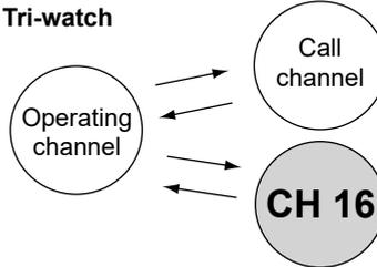
Periodically checks Channel 16 and the Call channel while operating on another channel.
