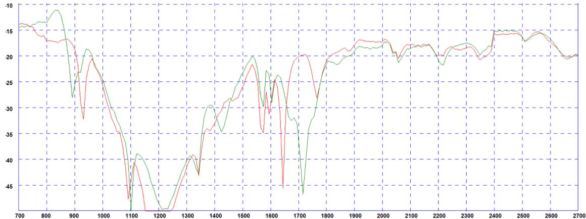
\*Isolation measured with no whip and 5m (16') of CS29 cable Green Plot = 600x600mm (2' X2') ground plane Red Plot = no ground plane
