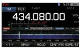
the high-speed spectrum scope, you can instantly see the operating band condition.
