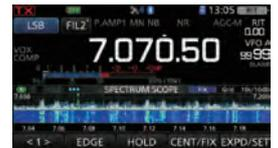
Display example of real-time spectrum scope and waterfall
